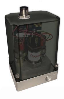
The Cordis is a closed-loop pressure control valve system designed to maintain a steady and repeatable downstream pressure under static conditions. Cordis comes in a IP65 rated enclosure for manufacturing and industrial environments. The unit is standard with two Clippard EV electronic valves designed for high pressure control.
